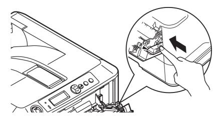
**3.** Ensure that the paper is loaded below the arrow level to avoid paper jam.
